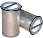
**WBPEL Series Basket-Type Filter Cartridge** with pleated polyester media and absolute rated at 99.9% efficiency. A Buna O-ring is provided in the top cap of the cartridge to prevent bypass. Flow is from inside to outside so as to capture particulates inside the basket for change-out through the top of the vessel without spillage. For **Type 65BT Dry Gas Filter** for removal of solid particles such as rust, scale, and dust.
