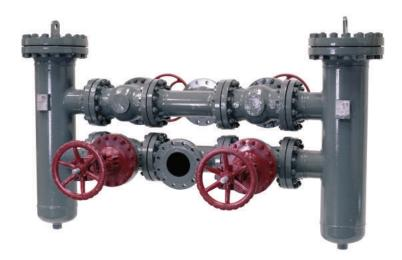
The Type **DU56** fabricated heavy duty duplex strainers are the solution to continuous operation when downtime is not an option. The assembly features two Type 56 strainers with modified inlet and outlet arrangements.
