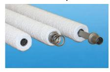
Fiber material such as cotton, polypropylene, or fiberglass is wound around a center core for the desired filtration needs. The core is offered in several materials to meet the application. Furnished separately, 304 stainless steel is the standard material for the installation hardware including the spring and cup assembly for the top hold down end and the post and pedestal for the bottom tube sheet end.
