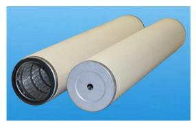
The fiberglass media tube, compressed to the desired density, is supported by a tinned steel core. A tinned steel end cap with bolt hole covers one end. Stainless steel is optional for core and end cap. The cartridge is wrapped externally with a cotton sock for protection during shipping and installation. Buna-N Gaskets are standard.
