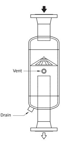
Type 120H-B Horizontal Flow With Boot for Liquid Collection
