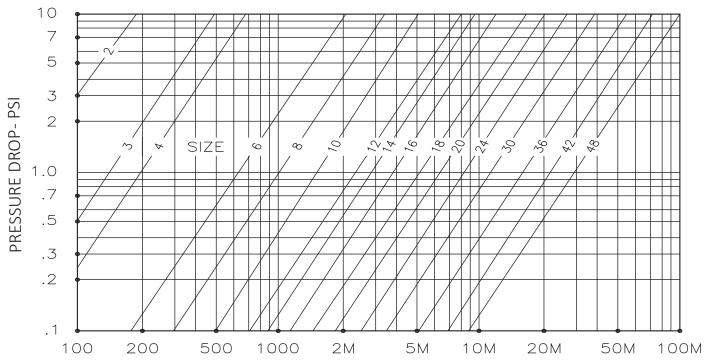
FLOW RATE OF WATER - GPM (CLEAN BASKET)
