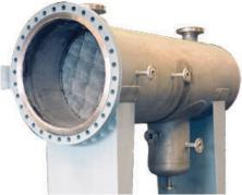
For each application the coalescer is designed for maximum dispersed phase liquid removal with minimal carryover. Variables which affect separation include velocity, viscosity, specific gravity, surfactants, and interfacial tension.
