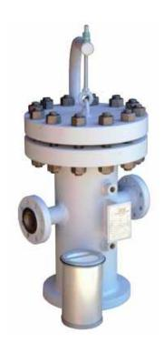
With the large surface area of the pleated design, the polyester cartridge provides the maximum dry contaminant holding capacity. The filter is an excellent choice for expected high solids loading and has a very low clean pressure drop. With a pleated design, the filter cartridge offers a longer service life between cartridge change-outs resulting in lower maintenance costs and increased operational efficiency.
