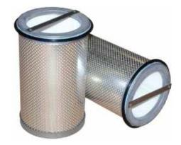
With this single open end cartridge, the solid particulates are collected in the interior of the filter basket for easy change-out through the top of the vessel housing without spillage. The polyester filter media is provided with tinned steel end caps. A Buna O-ring is provided in the top cap of the cartridge to prevent bypass.
