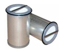
With this single open end cartridge, the solid particulates are collected in the interior of the filter basket for easy change-out through the top of the vessel housing without spillage. The polyester filter media is provided with tinned steel end caps. A Buna O-ring is provided in the top cap of the cartridge to prevent bypass.
