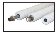
Fiber material such as cotton, polypropylene, or fiberglass is wound around a center core for the desired filtration needs. The core is offered in several materials to meet the application. Furnished separately, 304 stainless steel is the standard material for the installation hardware including the spring and cup assembly for the top hold down end and the post and pedestal for the bottom tube sheet end.
