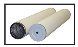
The fiberglass media tube, compressed to the desired density, is supported by a tinned steel core. A tinned steel end cap with bolt hole covers one end. 304 or 316 stainless steel is optional for core and end cap. The cartridge is wrapped externally with a cotton sock for protection during shipping and installation. Buna-N Gaskets are standard.
