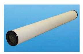
The media tube is made up of materials specifically designed to enhance the process of coalescence and is supported by a perforated metal core. A metal end cap with bolt hole covers one end. The cartridge is wrapped externally with a cotton sock for additional coalesced water drainage.
