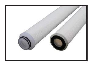
**Shown in the photo above** are two available bottom end treatments. On the left is style 222 with O-rings. On the right is a flat end, style FEG with gasket. Top end treatments are typically closed and with a spring assembly or a flat cap.
