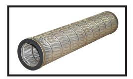
Providing a much greater surface area than a depth type filter, the pleated media cartridge is an excellent choice for expected high solids loading applications with the benefit of lower operating pressure drop and less frequent cartridge change-outs. For maximum efficiency these cartridges are rated to either 99.9% or 99.98% removal of 1 micron and larger solid particles.
